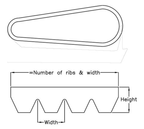
$\begin{array}{ll} \text{Datum Llength} = 2324 \\ \text{Height} &= 9.5 \\ \text{Number of ribs} = 16 \\ \text{Pitch} &= 4.7 \end{array}$
